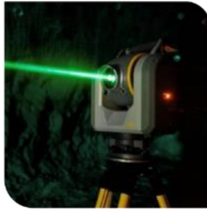
Total - station survey
